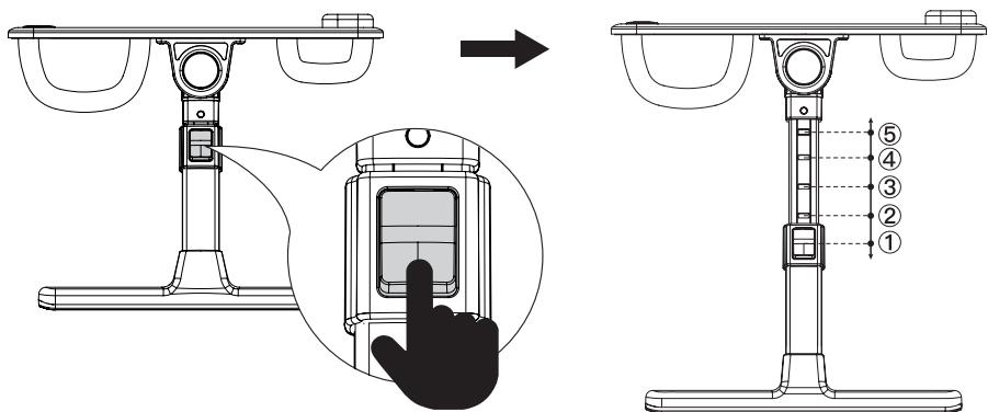
You can adjust the height of the work surface 5 times.
