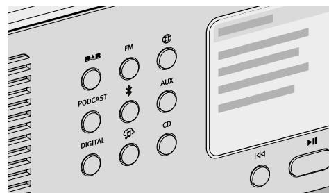
Select the playback source directly via the designated buttons on the unit.
