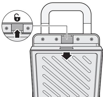
Each plate is secured in place by a locking catch in the device.
