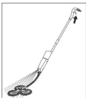
Pull the lever to activate the spray function!
