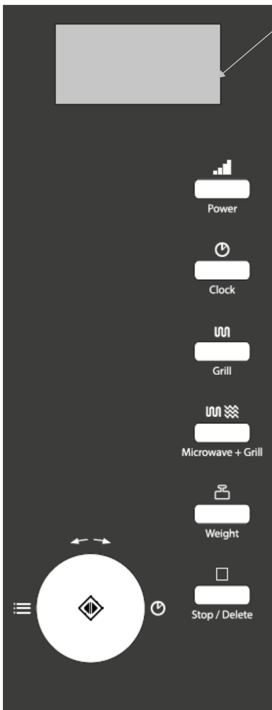
**Display panel:** Cooking time, output, function display and actual time are displayed.
