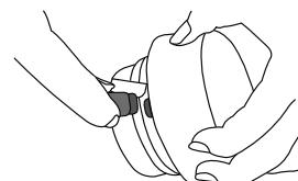
3. Insert the mains adapter into a suitable socket.
