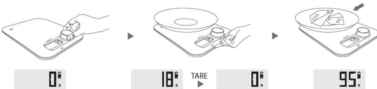
Place an empty container on the scale. The LED display will now show the weight of the container.
